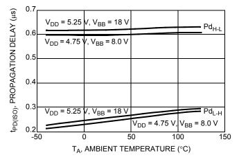
Figure 7. ISO Propagation Delay vs. Temperature
