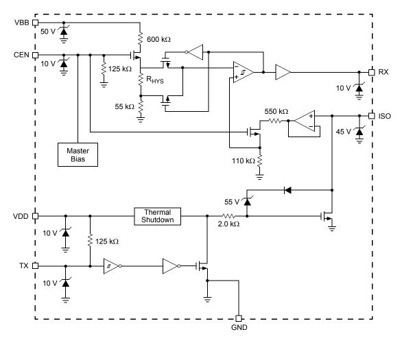
Figure 2. 33660 Simplified Internal Block Diagram
