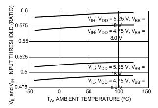
Figure 4. ISO Input Threshold/V<sub>BB</sub> vs. Temperature
