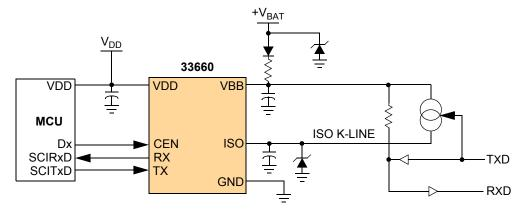
Figure 1. 33660 Simplified Application Diagram
